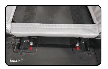
**STEP 6** Remove the driver seat bottom by pulling up on the front of the seat pan. Set aside. Using a 12mm socket, remove the four frame bolts as shown and remove frame assembly. NOTE: Retain these bolts for future use (*figure 5*).
