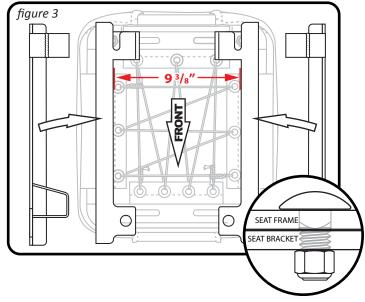
**STEP 4** Install the left and right passenger seat brackets as shown. Brackets should be spaced apart  $9\frac{3}{8}$ , centered on the seat frame. Secure with four nyloc nuts (figure 3).
